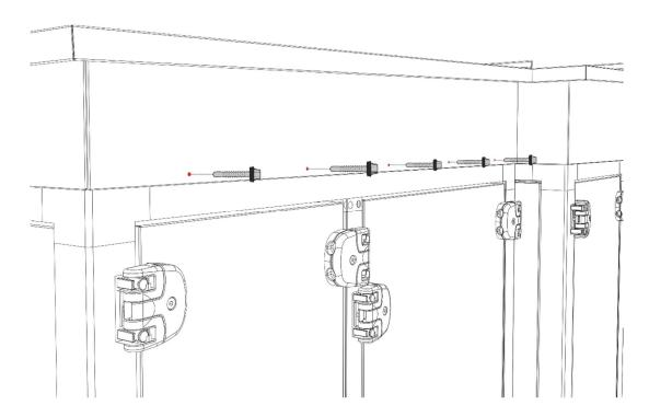
5. Paste silicone into metal U-shaped profiles. Put the profiles onto the connections of roof plates.
