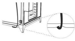
Rabbet for leading the rope when tying up the block from underneath
