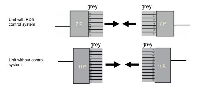
Rotary heat exchanger – connect red and grey connector above the middle block
