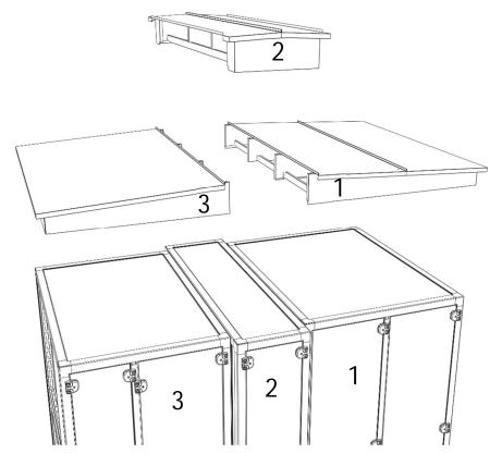
3. Fix the roof blocks together, use 8 screws M6, place waterproof washers (part of delivery) under the screws.
