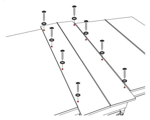
4. Attach side plates of roof blocks to the side of unit casing. Use holes that are drilled in the side plates. Use tek screws star 4x16mm (part of delivery). Attach the tek screws directly into the casing all around the unit.
