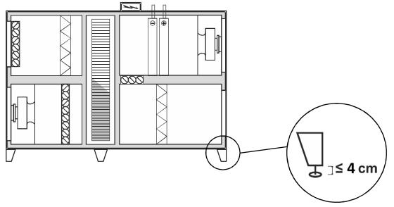
The base frame of the unit must not be disassembled or modified in any way – there is a risk of mechanical damage to the unit.
